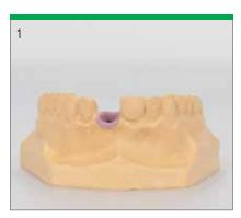
Fabricate the master cast including a gingival mask.
